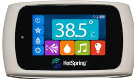
The Hot Spring Wireless Control Panel features a full color LCD touchscreen to operate all spa functions and features, wireless communication to the control system, and wireless charging via the bartop docking tray.
