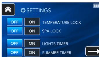
The first Settings screen allows you to turn Temperature Lock, Spa Lock, Lights Timer and Summer Timer On or Off.
