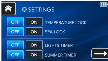
When activated, the exterior lights of the spa will come on 5 seconds later will remain lit for 6 hours and repeat the cycle every 24 hours from activation time.
