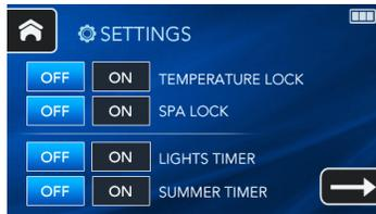
The Temperature Lock feature prevents changing the desired water temperature setting. All other control panel functions will operate normally while the Temperature Lock is "ON".
