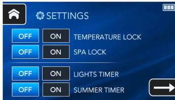
When activated, the Spa Lock feature disables all functions on the control panel.
