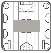
When using a cart below hot tub, entire center of hot tub must be supported as illustrated
