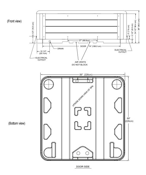
**NOTE:** Watkins Manufacturing Corporation recommends that the *Pulse* be installed on a minimum 10cm thick reinforced concrete pad or structurally sound deck able to support the "dead weight" found in the hot tub specification chart.
