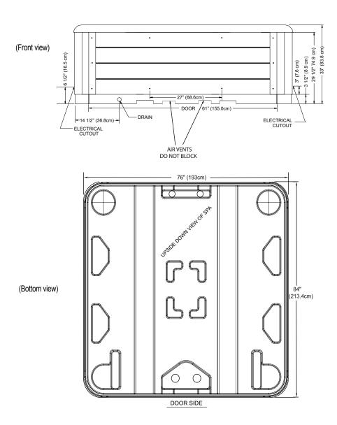
**NOTE:** Watkins Manufacturing Corporation recommends that the *Glow* be installed on a minimum 10cm thick reinforced concrete pad or structurally sound deck able to support the "dead weight" found in the hot tub specification chart.
