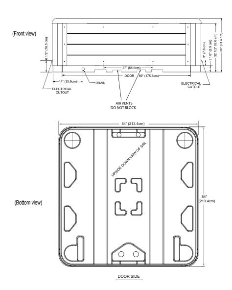
**NOTE:** Watkins Manufacturing Corporation recommends that the *Flair* be installed on a minimum 10cm thick reinforced concrete pad or structurally sound deck able to support the "dead weight" found in the hot tub specification chart.
